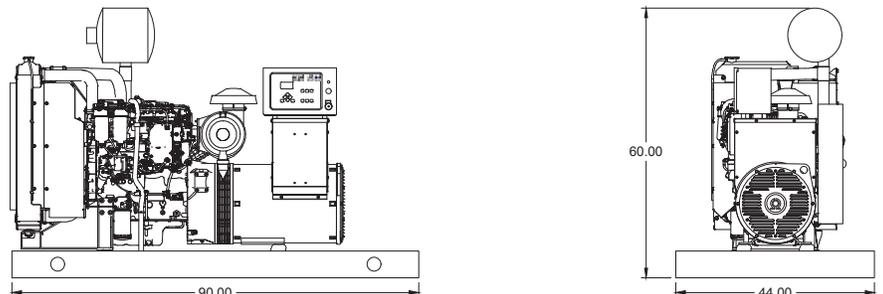
Drawings based on standard open power 480 volt standby generator. Lengths may vary with other voltages. Subject to change without notice. Sound data as measured at 23 feet (7 meters) in accordance with ISO 8528-10 at standby rating.
