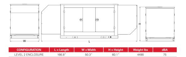
\* All measurements are approximate and for estimation purposes only. Weights are without fuel tank. Sound levels measured at 23ft (7m) and does not account for ambient site conditions.
